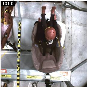
Test # 4: Thin, Wedge, Soft, 16°; Head X = 352 mm from normally seated
