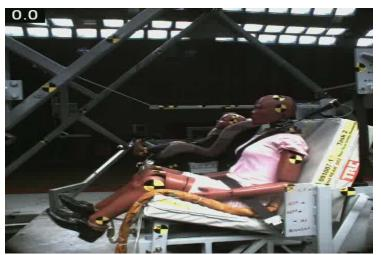
Test # 2: Thin, Wedge, Hard, 16°; Head X = 414 mm from normally seated
