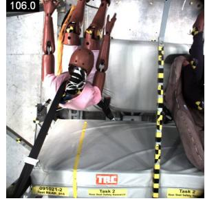
Test # 2: Thin, Wedge, Hard, 16°; Head X = 414 mm from normally seated
