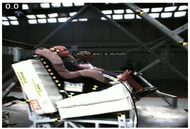
Test # 9: Thick, Wedge, Soft, 16°; Head X = 433 mm from normally seated
