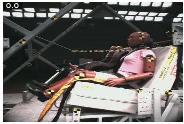
Test # 16: Thick, Flat, Hard,  $16^{\circ}$ ; Head X = 472 mm from normally seated
