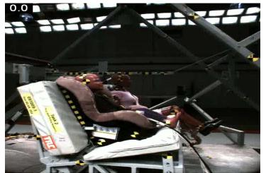
Test # 4: Thin, Wedge, Soft, 16°; Head X = 352 mm from normally seated
