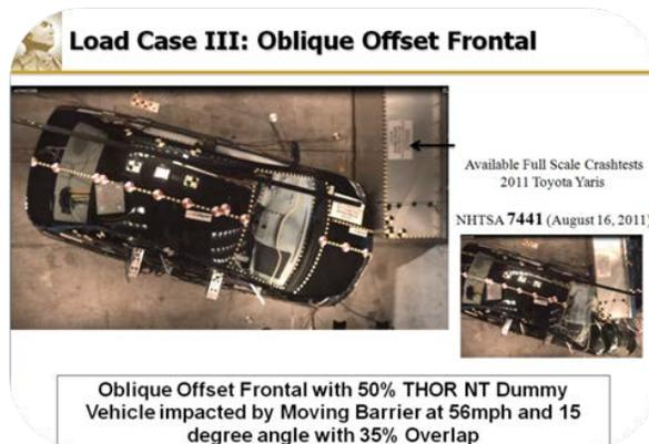
**Figure 13: Oblique offset frontal configuration**
