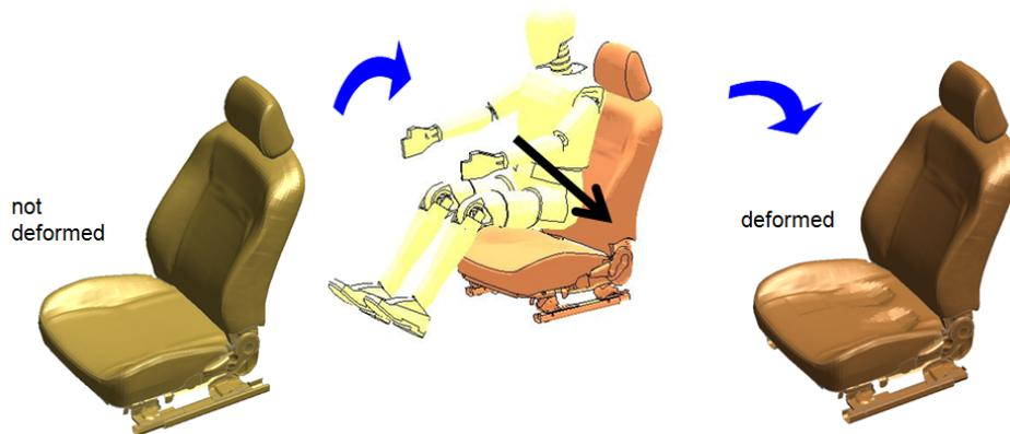
**Seat Squash: Simulation with Rigidified Dummy and Prescribed Motion into final Seating position is used to create “squashed” Seat**
