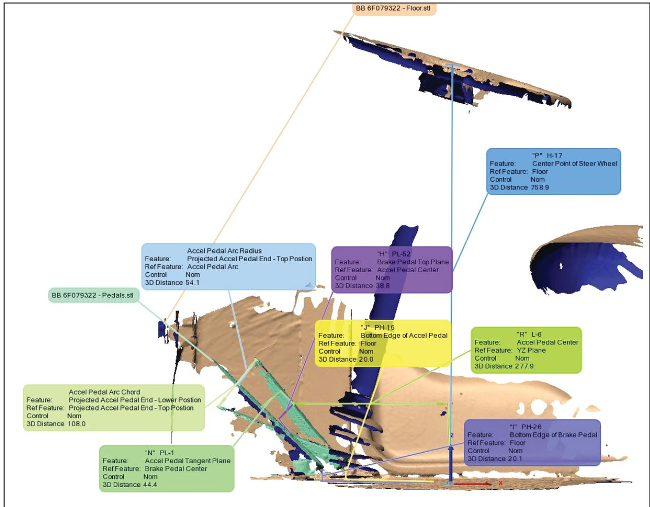
**Figure 4 - Dimensions H, J, N, P, R, Pedal Arcs**
