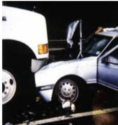
The impact occurred at a Delta V of 60 kph (33 mph) with a maximum crush of 76cm at C6. There was a major degree of bumper override of the delivery truck with the sedan, so that the engine was driven back toward the passenger compartment with intrusion of the steering wheel into the driver's space (Figure 8).
