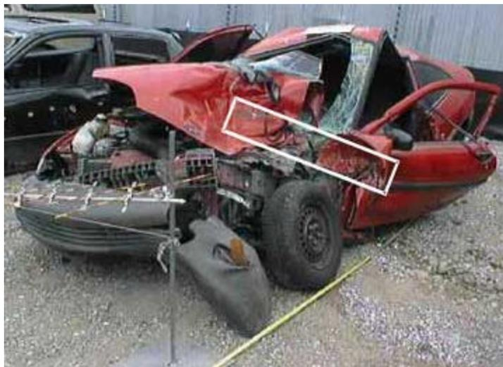
Frontal offset impact showing mismatch and override of the vehicle frame of a passenger vehicle (shown here) by the higher bumper frame of a light truck vehicle. The white rectangle indicates the position of the bumper of the light truck vehicle.
