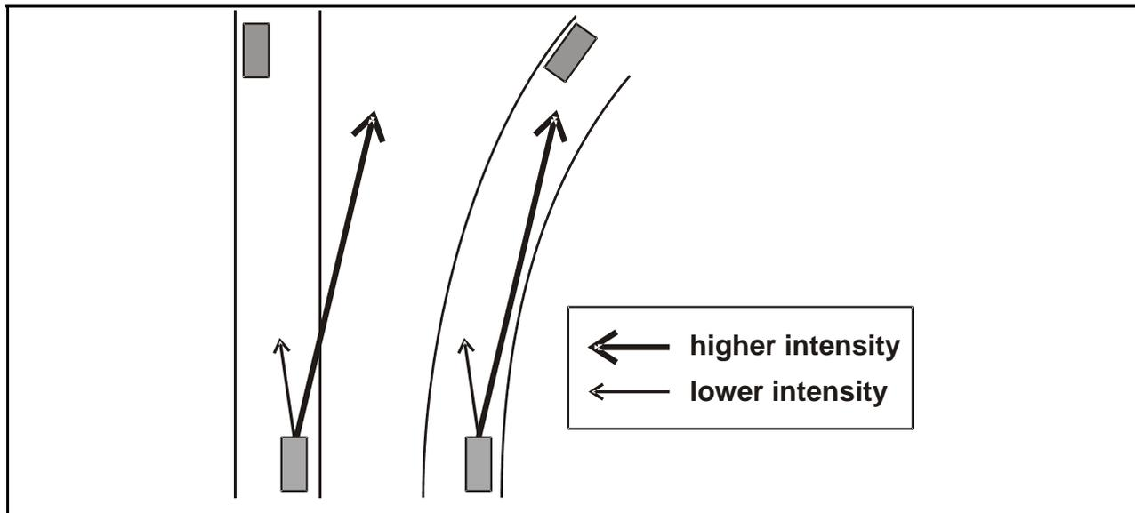
Figure 3. The effect of a curve on oncoming traffic glare exposure.
