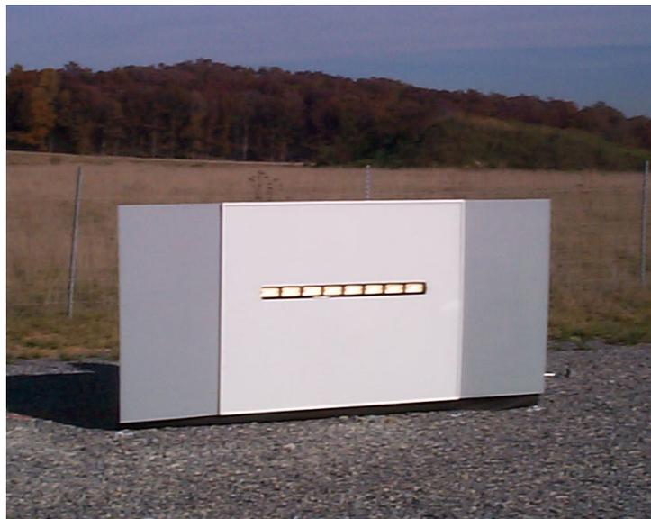
**Figure 12. Test configuration D: eight lamp bar with all eight lamps on continuously. (Note that actual brightness was greater than it appears in this photo.)**
