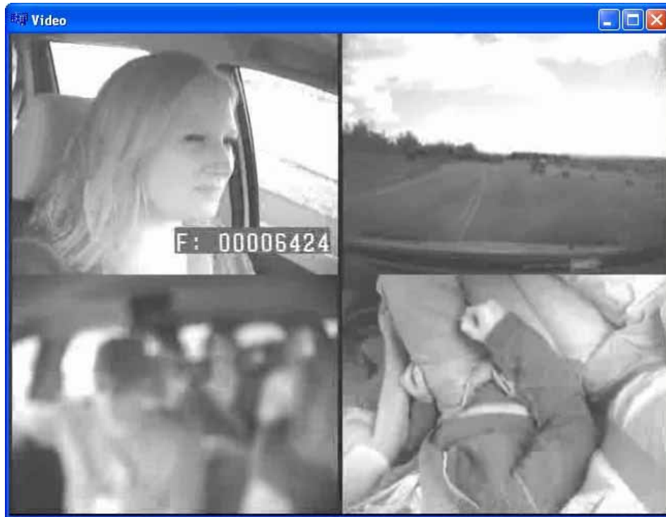
Figure 2. The quad image with two continuous cameras on the top two locations with the still frames in the two bottom locations. From upper left to right: driver face view, forward view, the blurred image of the vehicle cabin, and the back seat passenger lap camera
