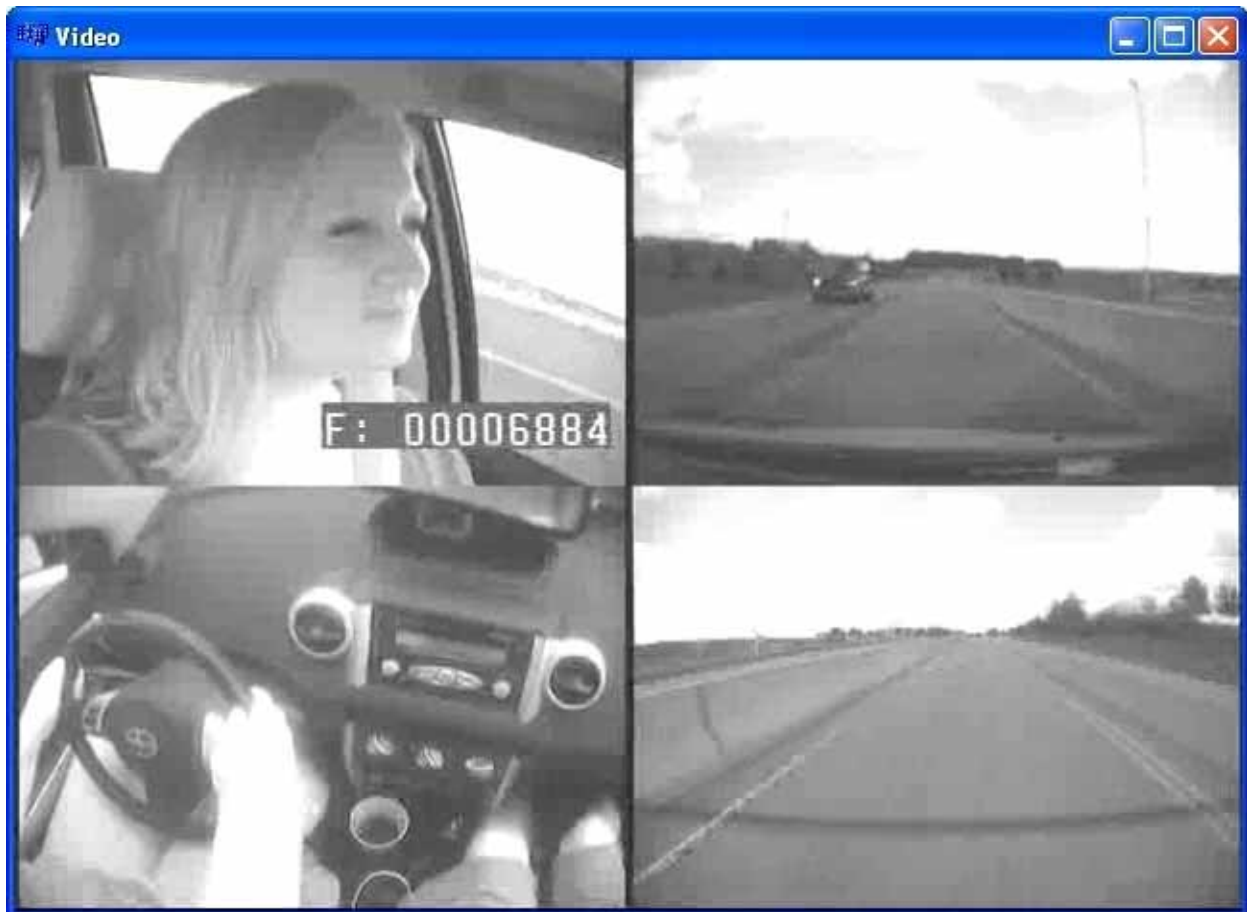
Figure 6. The Quad-image of the Four Continuous Video Camera Locations. From Upper Left to Right: Driver Face Camera, Forward View, Over-the-shoulder, and Rear-view.
