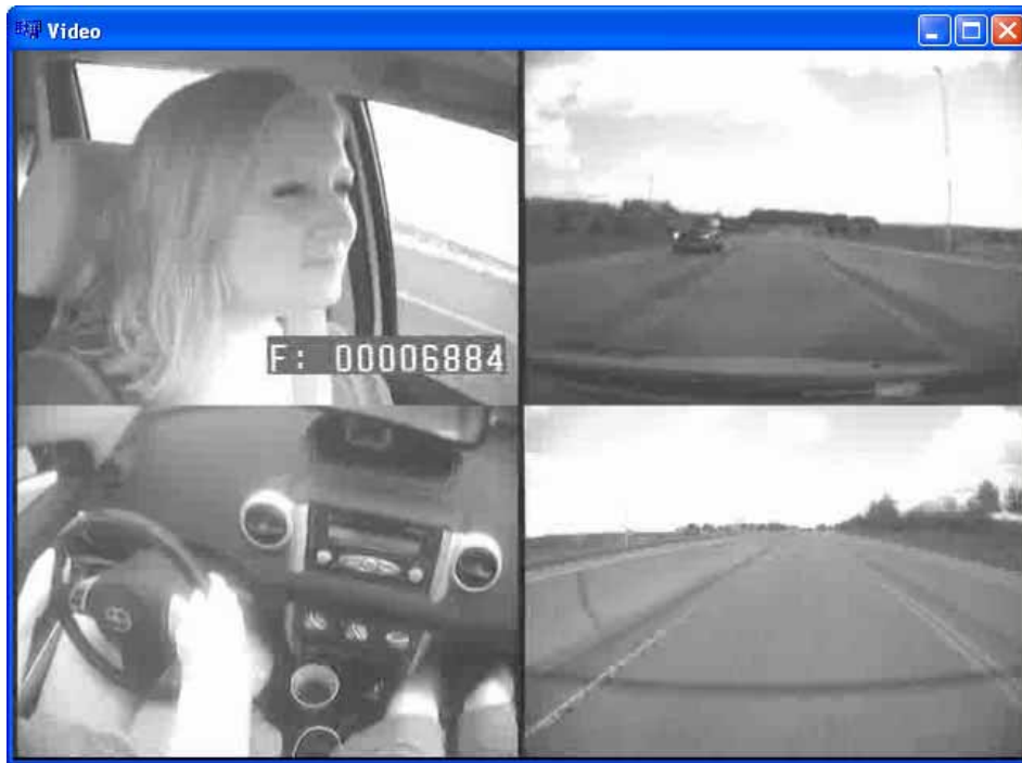
Figure 1. The quad-image of the 4 continuous video camera locations. From upper left to right: driver face camera, forward view, over-the-shoulder, and rear-view
