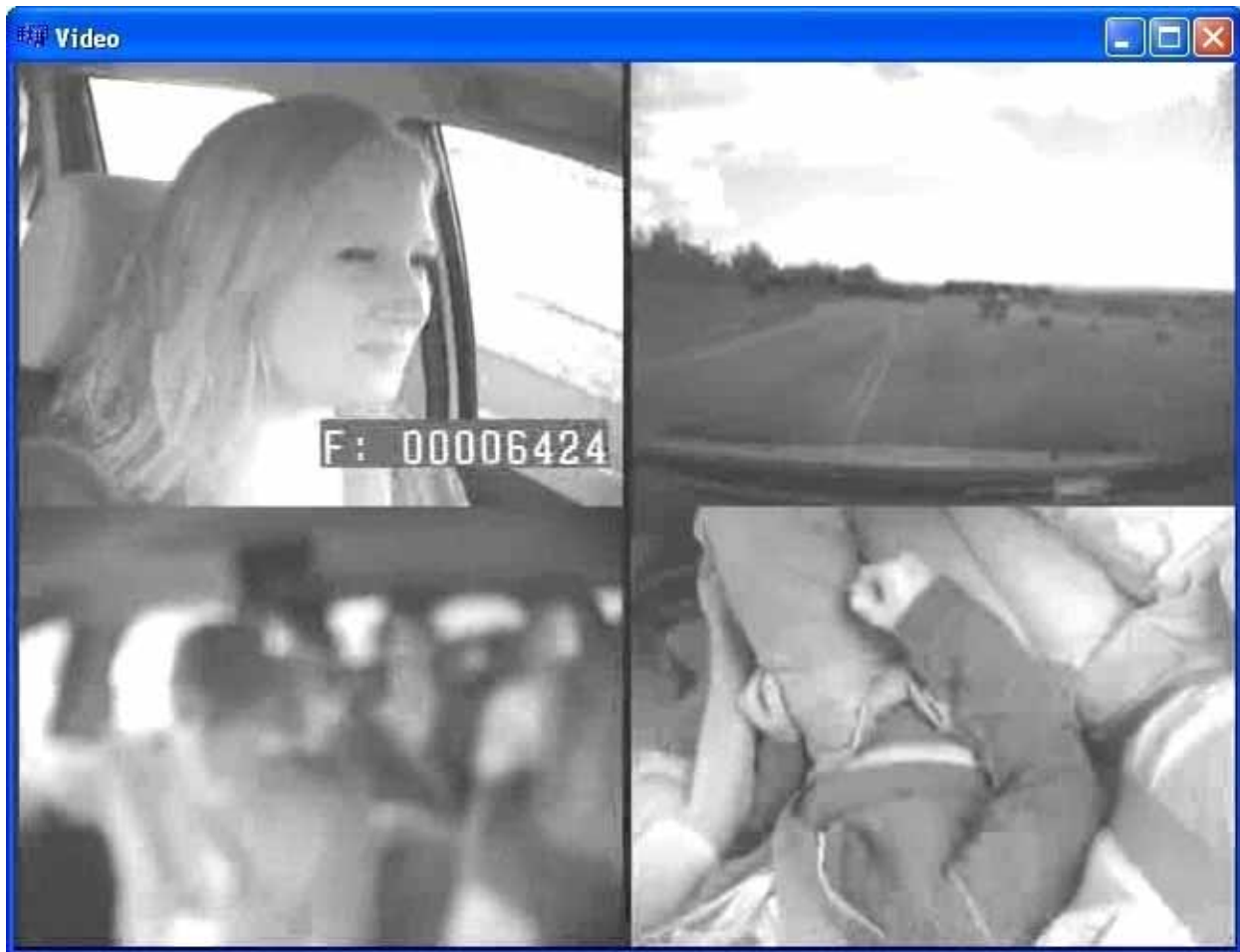
Figure 7. The Quad Image with Two Continuous Video Feeds on the Top Two Locations and Still Frames in the Two Bottom Locations. From Upper Left to Right: Driver Face View, Forward View, Blurred View of the Vehicle Cabin, and Back Seat Passenger Lap View.
