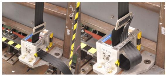
8. Route the webbing through the 3-bar clip, leaving about 5 inches of webbing tail. Route the tail end of the webbing back through the clip to lock it.
