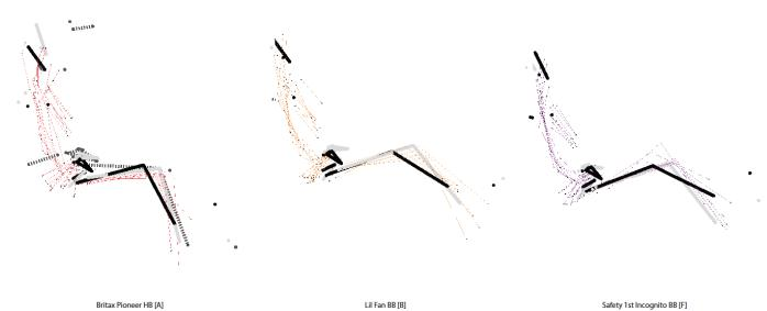
Figure C10. Comparison of postures of child volunteers with 10YO and small female across applicable booster configurations in TOYOTA vehicle. Cushion Length = 455 mm; Seat back angle = 26-deg; Cushion angle = 15-deg.
