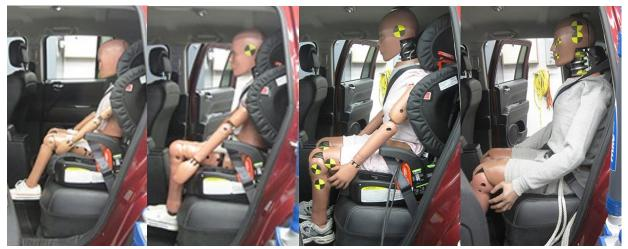
Figure 55. 6YO, 10YO, 5<sup>th</sup> ATDs on the Britax (A) and 50<sup>th</sup> on vehicle seat (left to right) in Jeep (vehicle with taller ceiling height)
