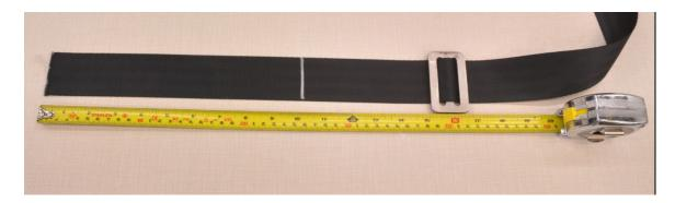
7. Thread the end of the webbing down through the split drum of the surrogate retractor until the 250 mm mark is visible. Then direct the webbing tail under the top framing bracket along the right side of the spindle.
