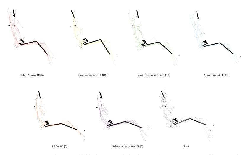
Figure C3. Comparison of postures of child volunteers overlaid and expressed w.r.t 6YO ATD across all booster configurations in B-L mockup. Cushion Length = 523 mm; Seat back angle = 23-deg; Cushion angle = 14.5-deg.
