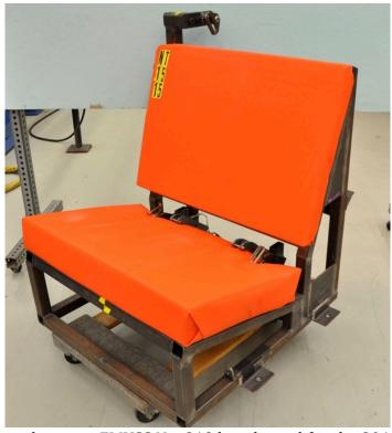
Figure 1. The preliminary FMVSS No. 213 bench used for the 2015 test series.
