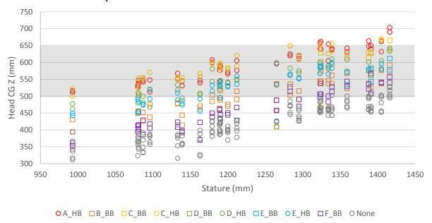
Figure 66. Head CG vertical location versus subject stature, relative to target zone defined by locations of small female and midsize male ATDs.
