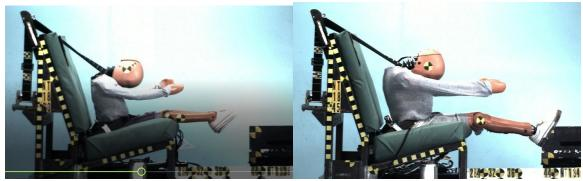
Figure 67. No-booster condition with 6YO (left) and 10YO (right) shows submarining tendencies on 2018 version of the bench.
