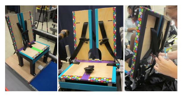
Figure 17. Hardseat used for measuring subject reference landmarks.
