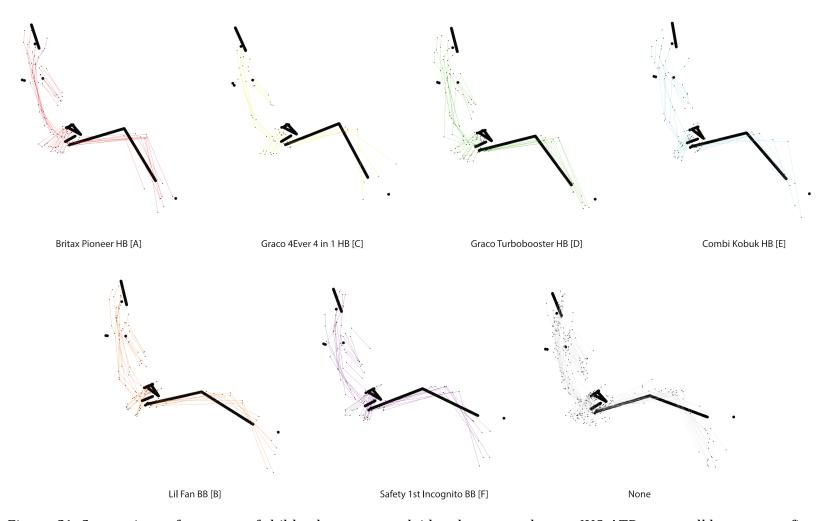
Figure C1. Comparison of postures of child volunteers overlaid and expressed w.r.t 6YO ATD across all booster configurations in B-Z mockup. Cushion Length = 465 mm; Seat back angle = 23-deg; Cushion angle = 14.5-deg.
