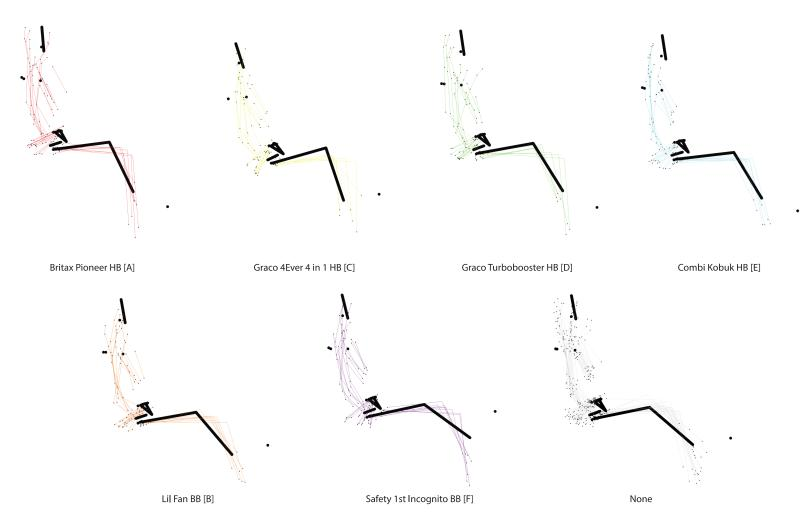
Figure C5. Comparison of postures of child volunteers overlaid and expressed w.r.t 6YO ATD across all booster configurations in JEEP vehicle. Cushion Length = 468 mm; Seat back angle = 22.5-deg; Cushion angle = 4-deg.
