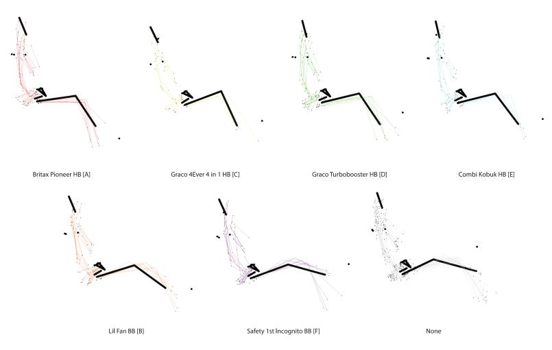
Figure C6. Comparison of postures of child volunteers overlaid and expressed w.r.t 6YO ATD across all booster configurations in MALIBUU vehicle. Cushion Length = 475 mm; Seat back angle = 23-deg; Cushion angle = 13-deg.
