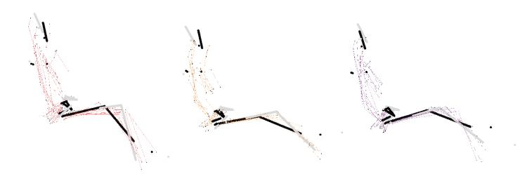
Figure C9. Comparison of postures of child volunteers with 10YO and small female across applicable booster configurations in B-L mockup. Cushion Length = 523 mm; Seat back angle = 23-deg; Cushion angle = 14.5-deg.
