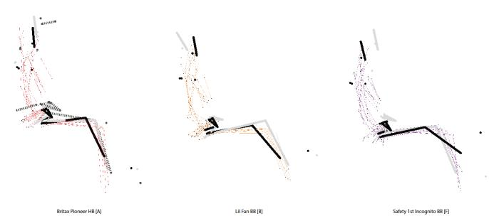
Figure C11. Comparison of postures of child volunteers with 10YO and small female across applicable booster configurations in JEEP vehicle. Cushion Length = 468 mm; Seat back angle = 22.5-deg; Cushion angle = 4-deg.
