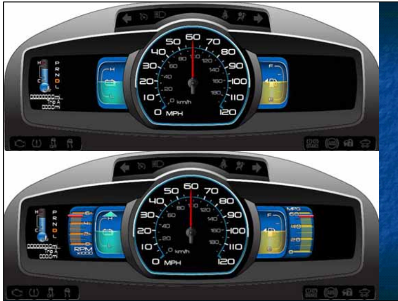
Figure 12. Example 8: Hybrid vehicle, user configurable displays
