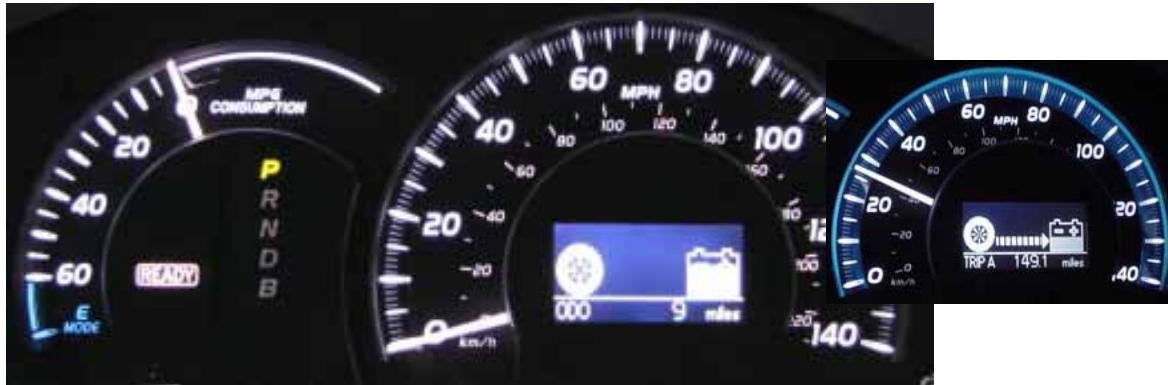
Figure 22. Toyota Camry hybrid (2009) instrument cluster with current fuel economy gauge and multi-information display
