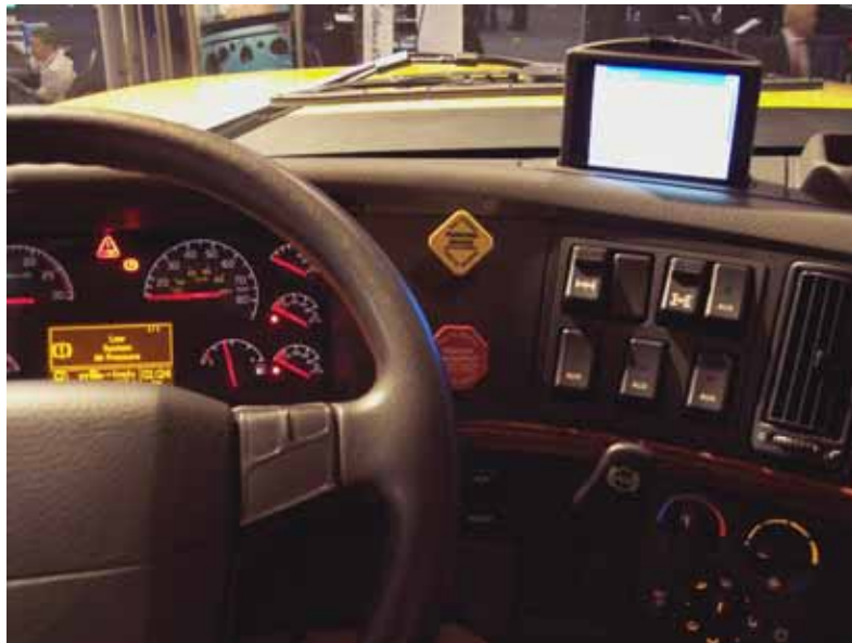
Figure 37. Volvo truck dashboard with multifunction display
