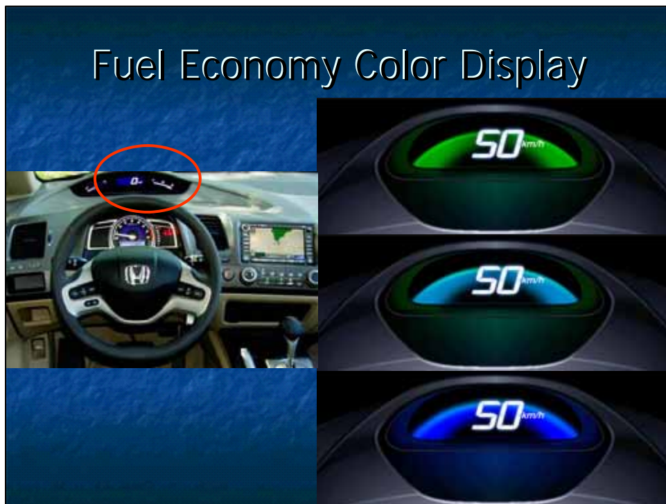
Figure 5. Example 2: Fuel economy colored arc display
