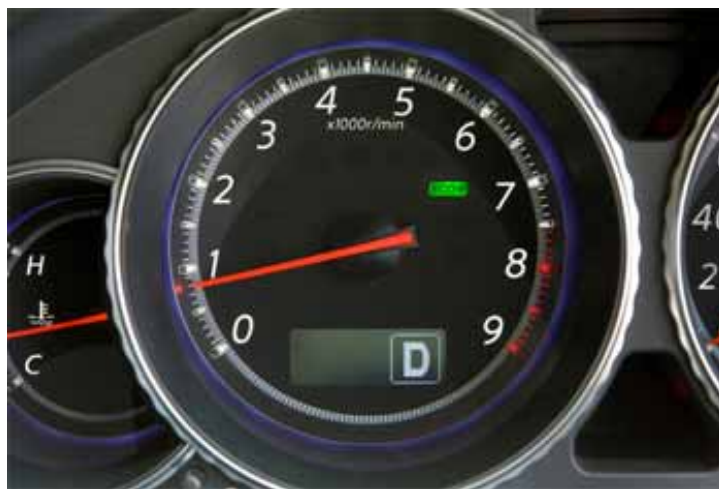
Figure 27. ECO indicator light
