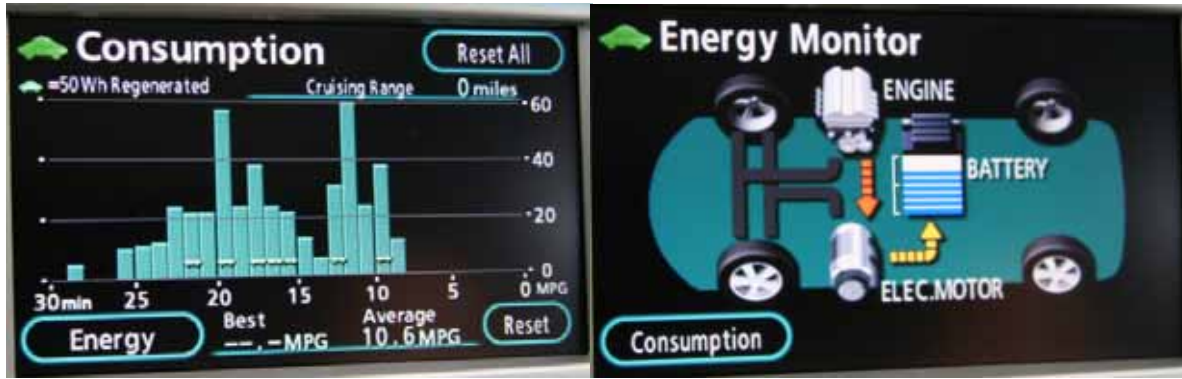
Figure 21. Toyota Camry hybrid (2009) consumption display (L) and energy monitor (R)
