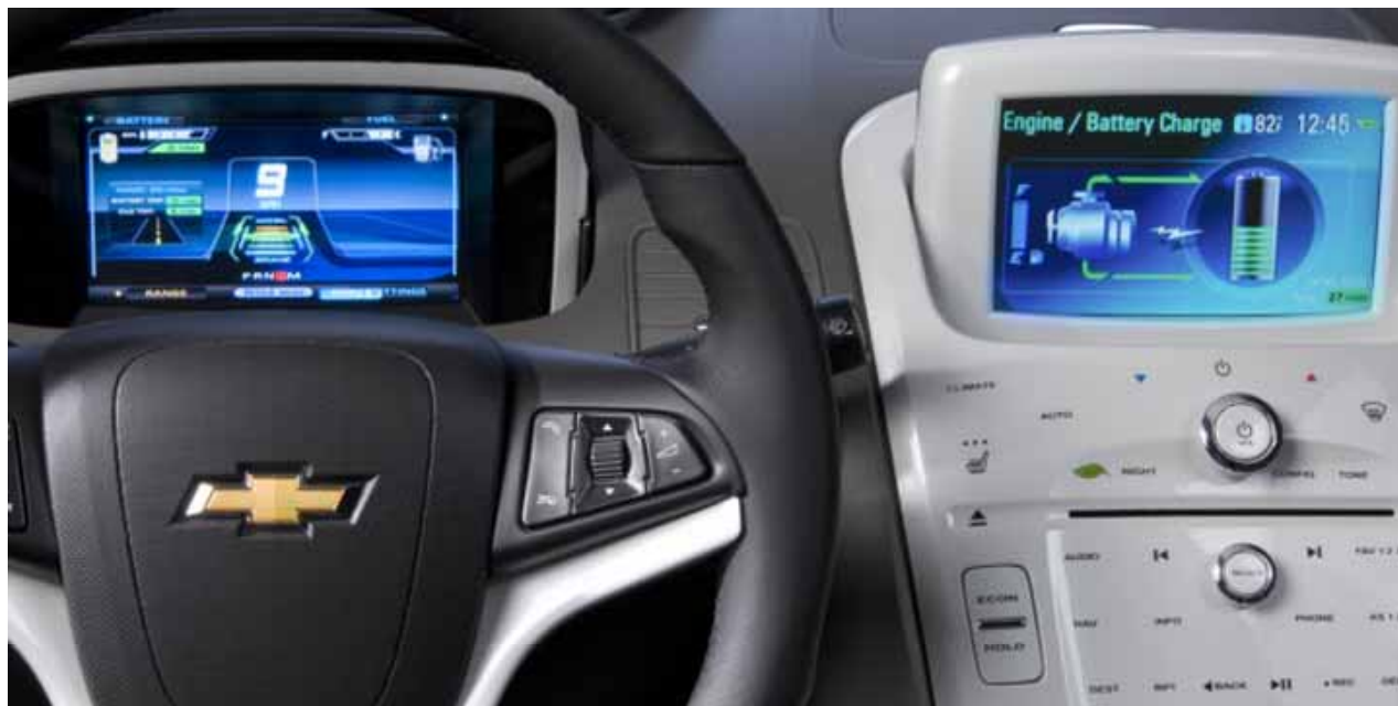
Figure 2. 2011 Chevy Volt dashboard and center console touch screen display (pre-production)
