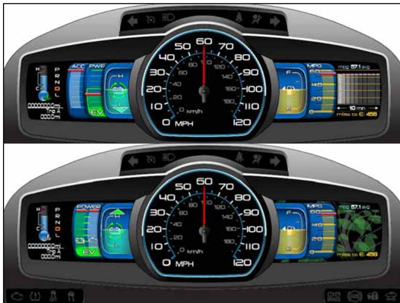
Figure 13. Example 8: Hybrid vehicle, graph and leaf displays
