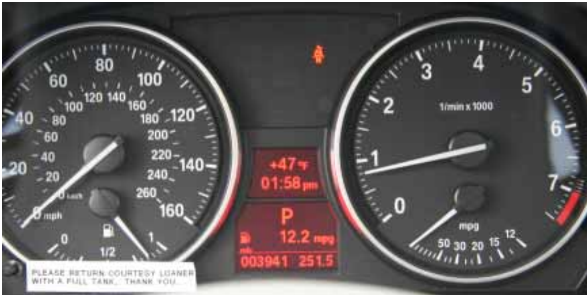
Figure 15. BMW fuel economy display with analog gauge (2008 328i)
