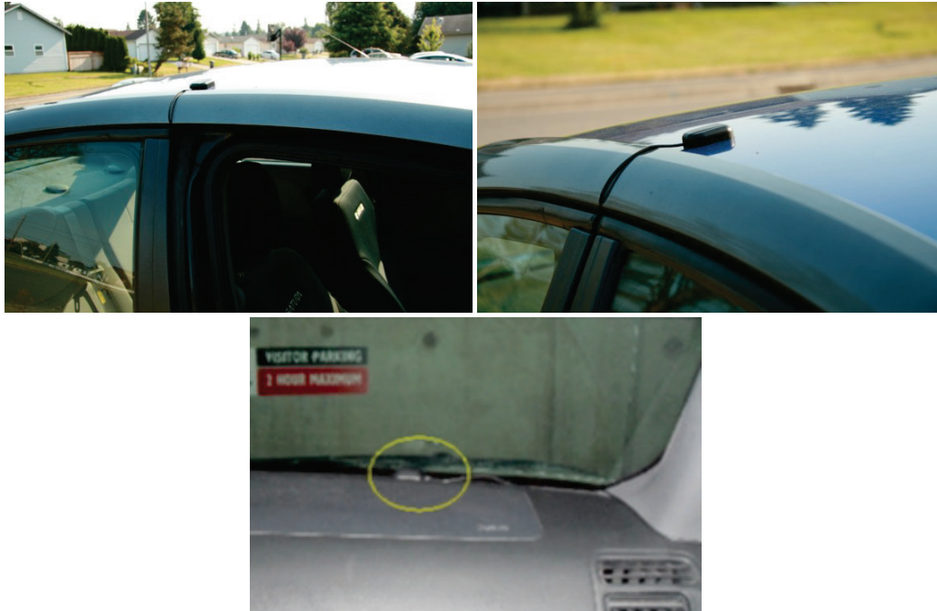
Figure 6. GPS installations using exterior and interior antenna mount options.
