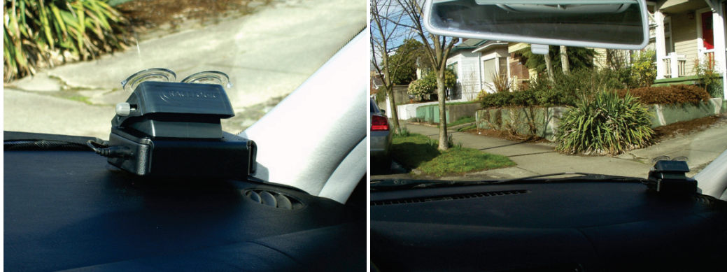
Figure 4. GPS installation using the windshield mount option.
