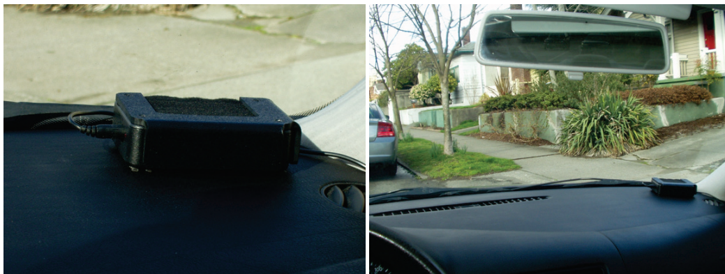
Figure 5. GPS installation using the dash mount option.
