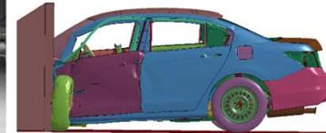
Post-test laboratory vehicle and model of the 2009 Honda Accord for IIHS SOL test
