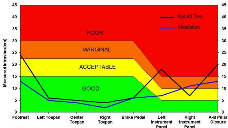
Maximum intrusion in laboratory test and finite element simulation in IIHS SOL frontal impact.
