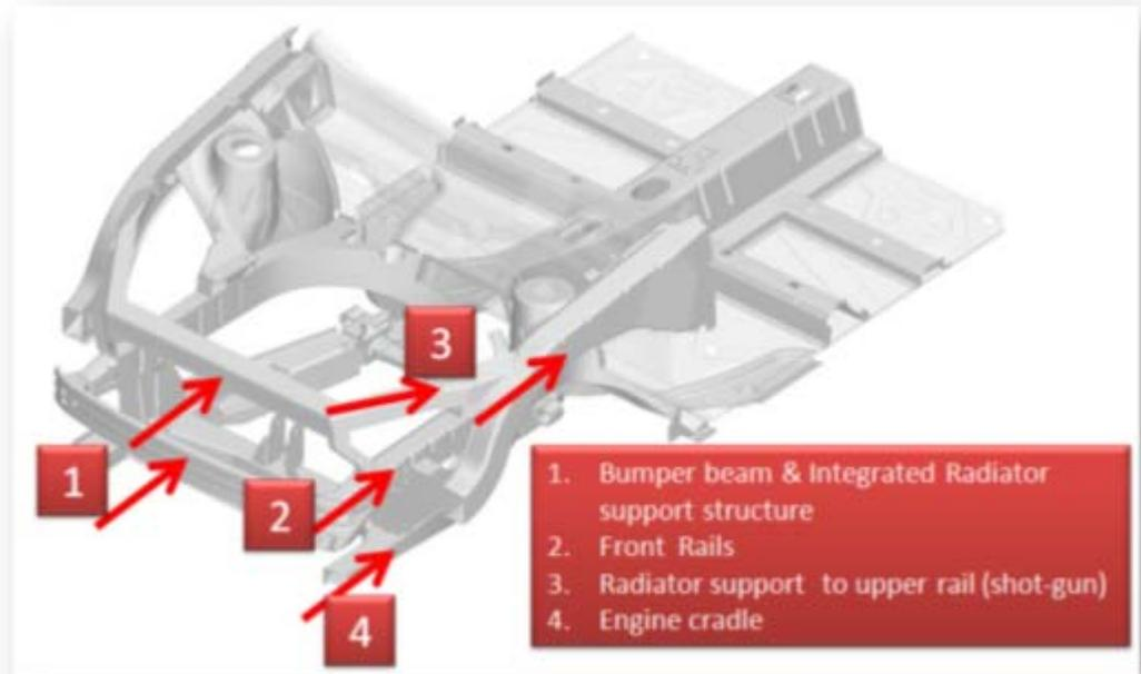
Figure 89: LWV Front Structure Load Paths
