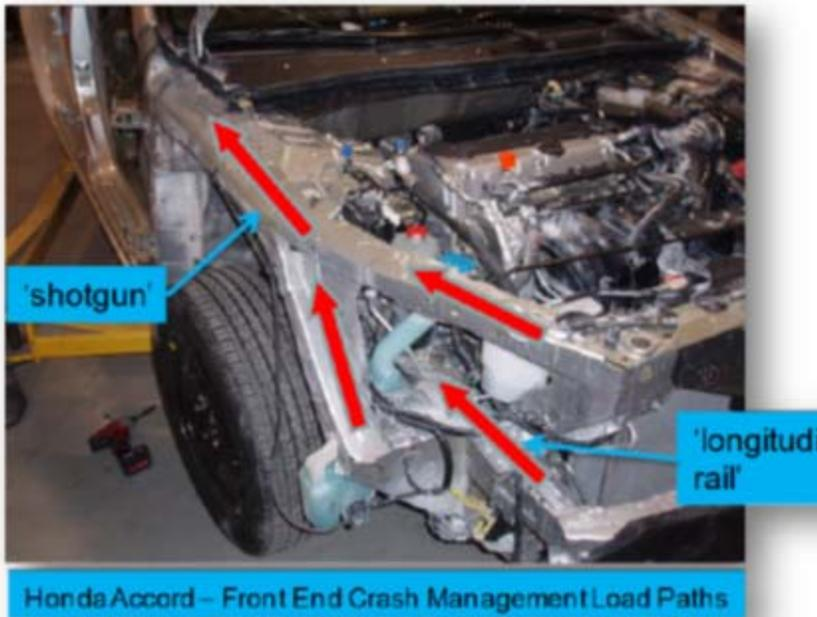
Figure 88: Honda Accord Front Structure
