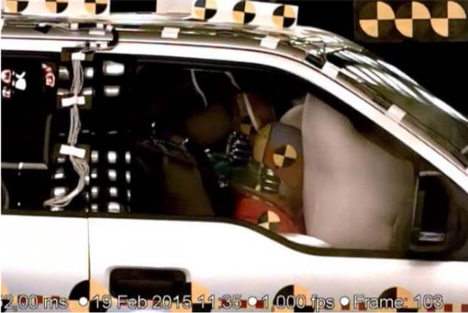
Ford F-150, test #9335, air bag deployment at 0.052 seconds
