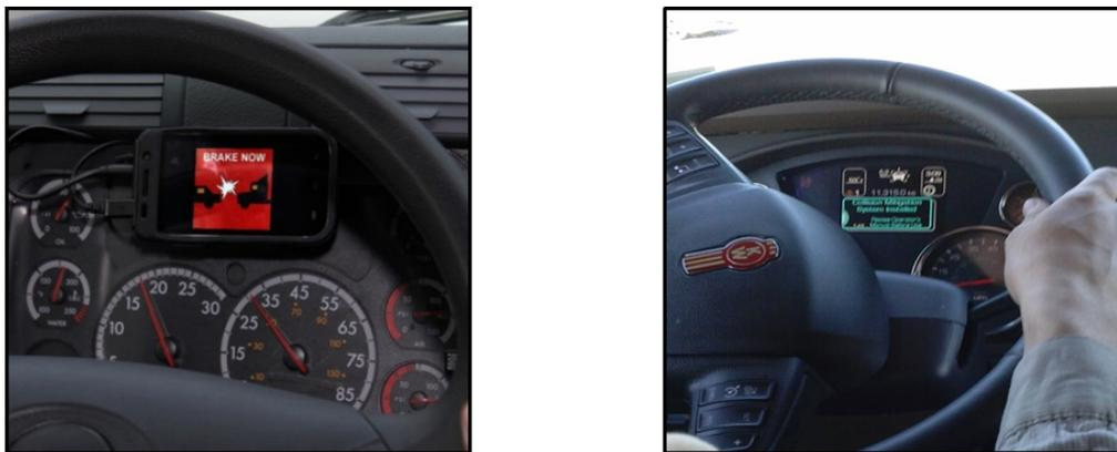
**Figure 8. Placement Comparison with OEM FCW System (in Green) in the Right Image**
